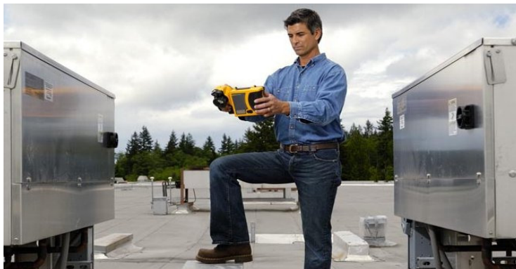
Figure 3. Figure 3: Qualitative measurements are fast for ducting, but accurate, quantitative measurements require compensating for reflectivity.
