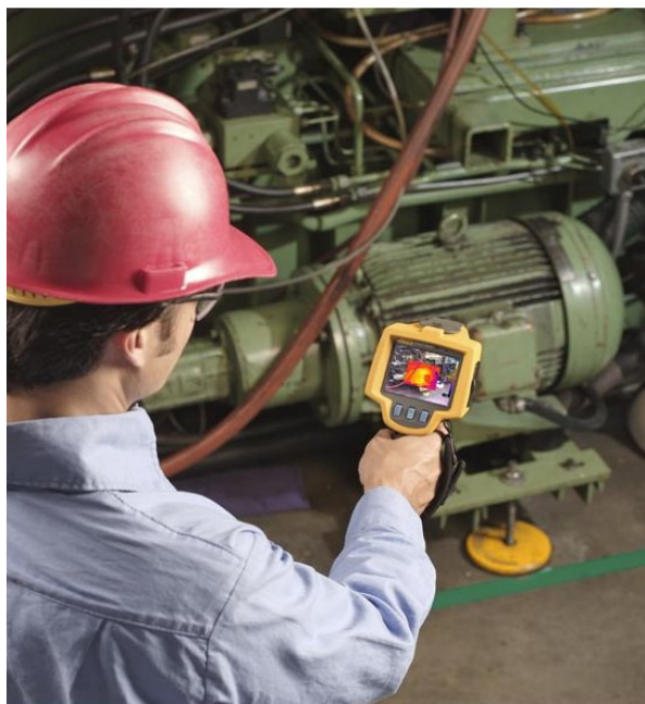
Figure 1. Thermal imagers offer a quick way to inspect equipment for abnormally hot-spots, and piping for abnormally cool spots.
